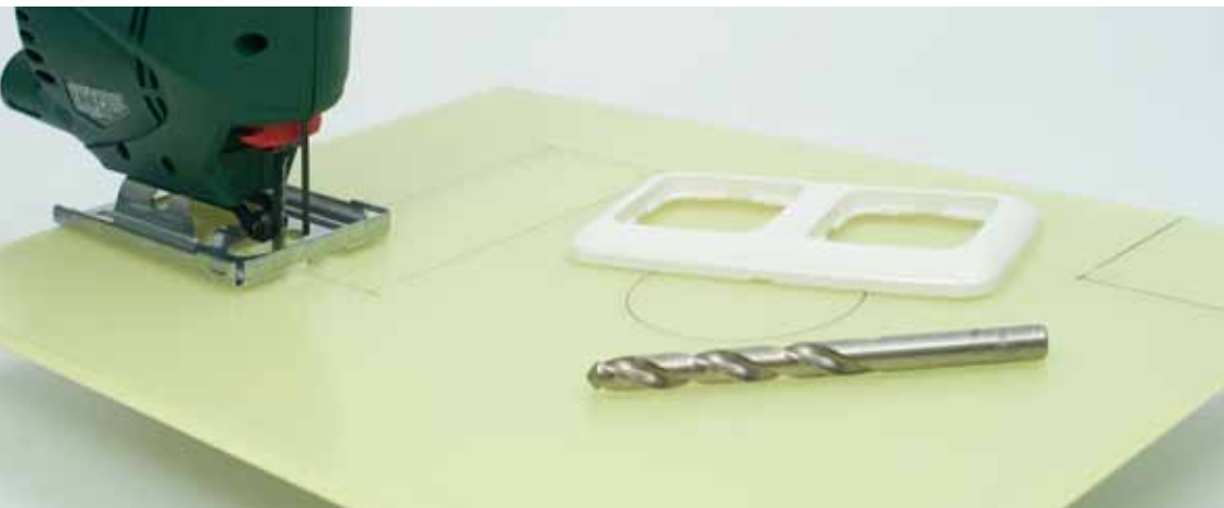
Always predrill recesses and apertures in the corners of cut edges and cut them out with a jigsaw or overhead template router.
