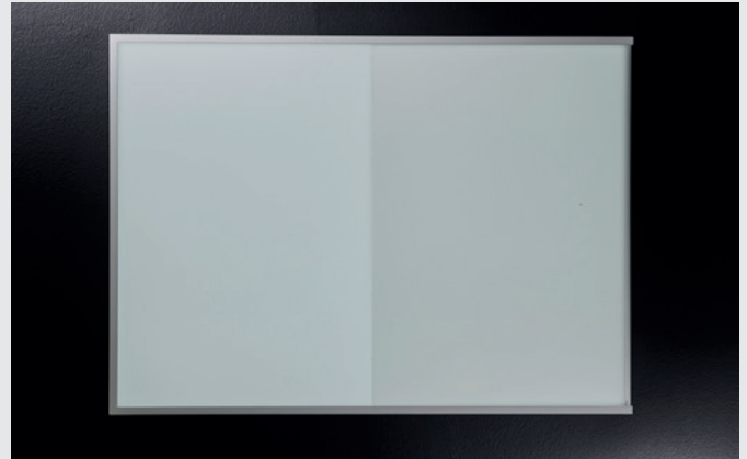
Fig. 2: Comparison of white tone by daylight (not illuminated) normal translucent white in signage (right): PLEXIGLAS® LED Pure White WH52 (left)
