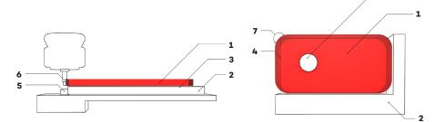
Fig. 26: Principle of overhead template routing (rounding of corners: 1 = workpiece, 2 = jig, 3 = stop, 4 = template, 5 = pilot pin, 6 = cutter, 7 = cutter working range, 8 = feed)
