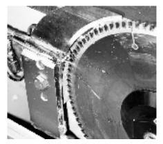
Fig. 5: Spray mist on circular saw blade
