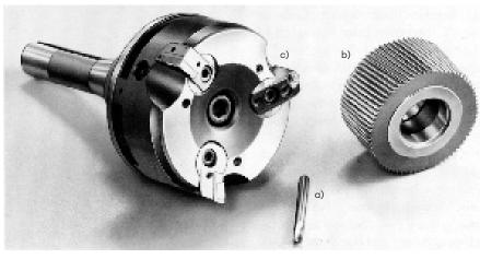
Fig. 24: Routing of PLEXIGLAS  $^{\otimes}$  with shell endmill; various other cutter types: (a) double-fluted cutter; (b) cylindrical cutter; (c) diamond cutter
