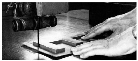
Fig. 7: Edge trimming with bandsaws
