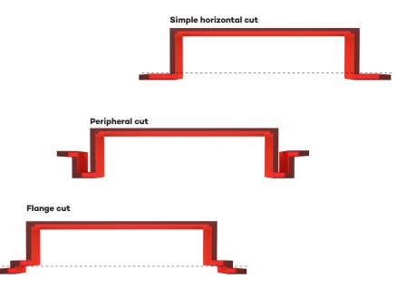
Fig. 8: Possible cuts with horizontal bandsaws
