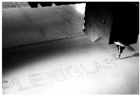
Fig. 27: Engraving with CNC portal-type machine; single-fluted graving bit.
