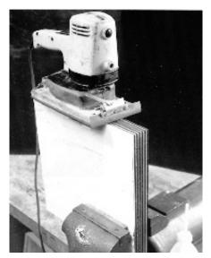
Fig. 37: Sanding the edge of a stack of blanks using an orbital sander
