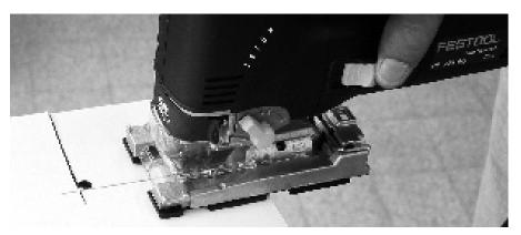
Fig. 10: Jigsawing after predrilling
