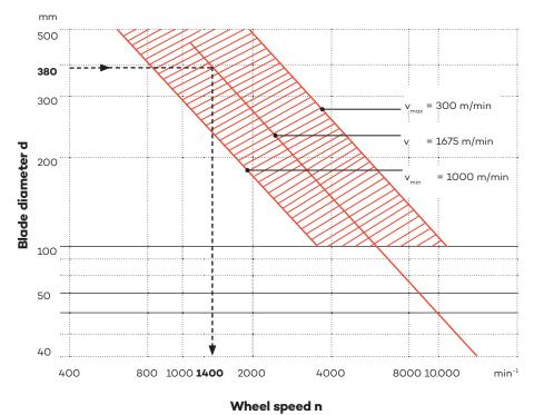
Fig. 6: Recommended cutting speeds, blade diameters, and wheel speeds for bandsawing of  $\mathsf{PLEXIGLAS}^{\otimes}$
