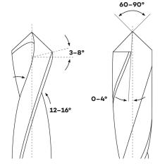
Fig. 12: Correct grinding of HSS drills for PLEXIGLAS® **(cutting edge must scrape**
