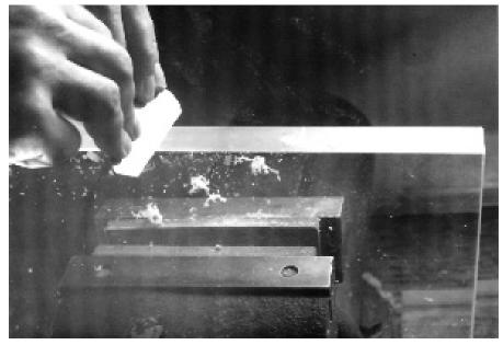
Fig. 35: Deburring PLEXIGLAS® with a scraper
