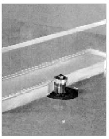
Fig. 21: Milling down beads of adhesive
