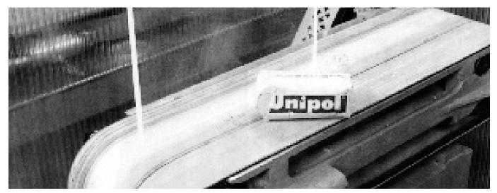
Fig. 39: Polishing against a felt belt
