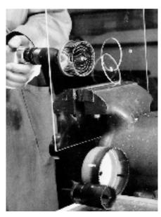
Fig. 17: "Slugger" cutter and hole saw
