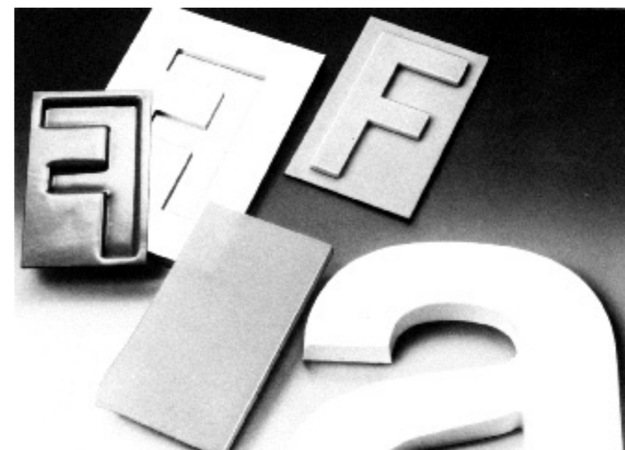
Fig. 20: PLEXIGLAS® GS letters pressure-formed using an aluminum mold and silicone rubber sheet
