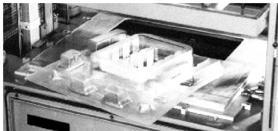
d: Removal of the molding
