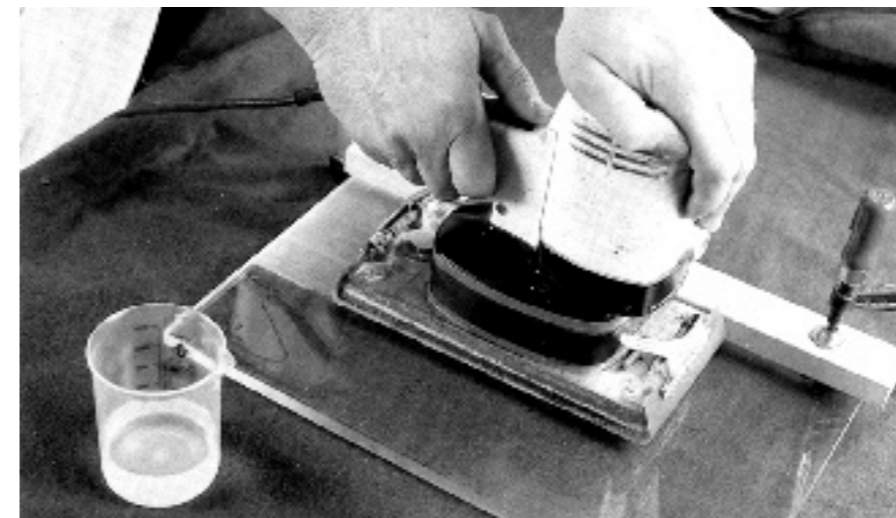
Figure 11: Mechanical matting with an orbital sander
