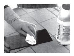
Figure 13: Chemical treatment of a previously sanded surface
