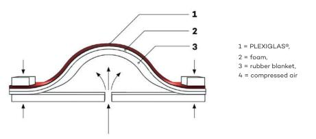
Figure 12: Schematic of blow molding of a light dome with matte interior surface
