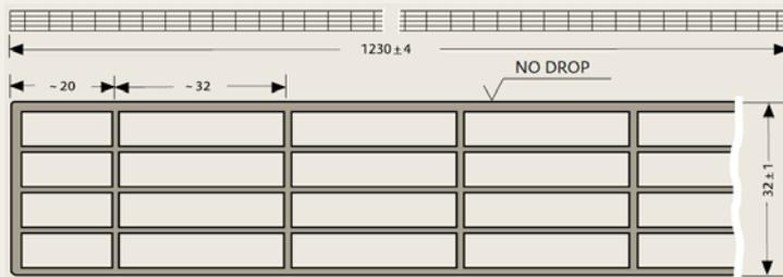
Cross-section of PLEXIGLAS® Heatstop Cool Blue S5P 32 (dimensions in mm)
