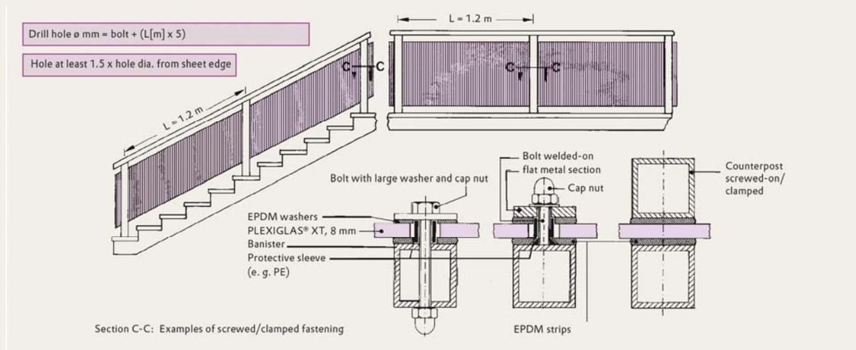
Fig. 11: Pointwise fastening
