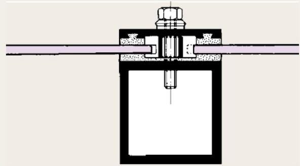
Fig. 6: Too high clamping pressure
