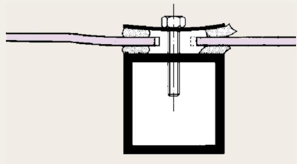
Fig. 7: Spacer sleeve
