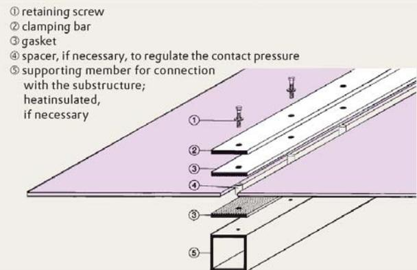
As a general principle, **linear fastening is to be preferred** since the load conditions are more favorable in this case and thinner sheets can be used as a result. The allowance to be made for expansion is again 5 mm/m for PLEXIGLAS® (PLEXIGLAS® Resist: 6 mm/m).
