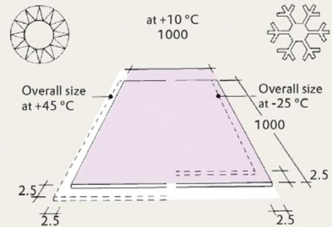
Because of the possible change in length, the clamping depth of the glazing should be between 15 and 20 mm. In addition, there is to be a clearance “a” for expansion and compensation for building tolerance. The value “a” depends on the sheet size and corresponds to one half of the general expansion allowance calculated as above (Fig. 2).
