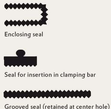
The sealing sections used determine the watertightness of glazing with PLEXIGLAS®. Particularly important is the material they are made of. PLEXIGLAS® is sensitive to certain sealants, which should therefore always be tested for **compatibility**.
