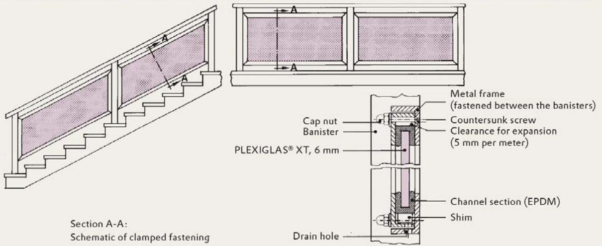
Fig. 9: Clamping on two sides
